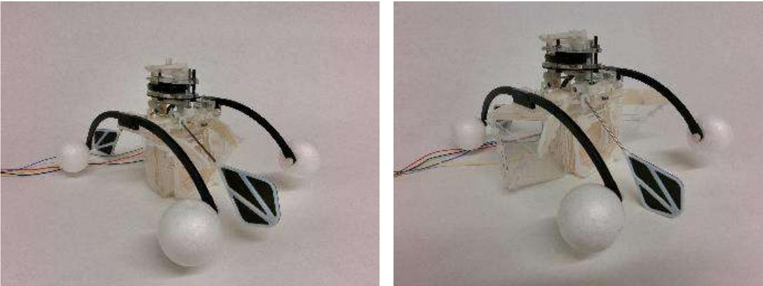
Soft body which is actuated to open and close as a mouth for allowing liquid food to flow in in order to be digested by the MFCs aboard
