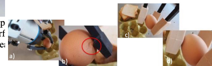
Fig. 18: View of the result of the first pick and place task using eggs. Confront between the broken egg resulted from the manipulation of the Festo grippers (a,b) and the same egg manipulated with silicon thimbles (c,d).
