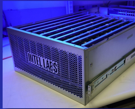
Pohoiki Springs system with 768 Loihi chips
